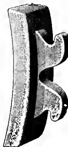
Figs. 5185-5186. THE SCHOEN PRESSED-STEEL BRAKE-SHOE.
